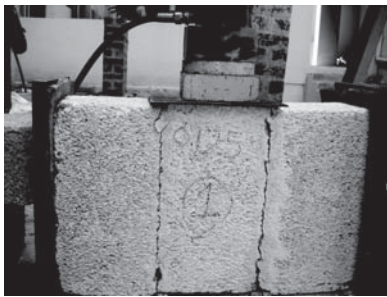
Fig.12 Observed failure Pattern of the concrete block triplet
