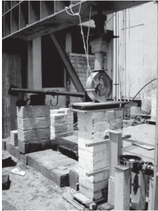
Fig. 2 Flexure test set up with the brick masonry wallette specimen
