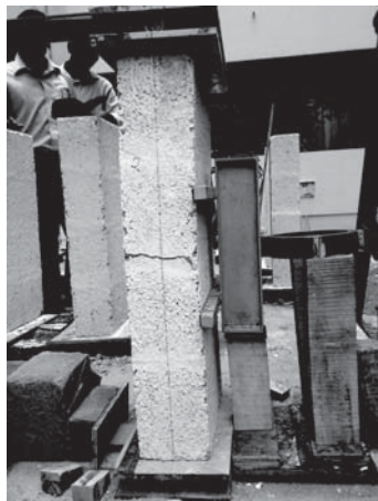
Fig. 8 Observed failure pattern of the concrete block masonry prism
