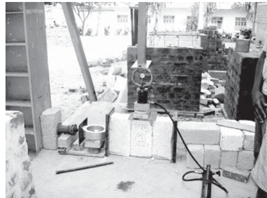
Fig. 5 Shear test set up for the concrete block triplet
