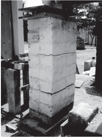
Fig. 7 Observed failure pattern of the one-brick thick masonry wallette
