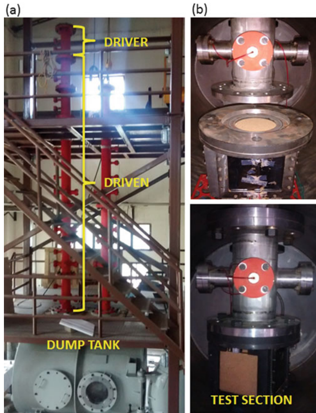
Fig. 1 (a) Complete assembly of vertical shock tube and (b) test section at the open end of the driven section
