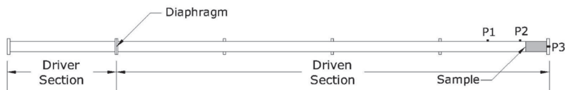
Fig. 2. A schematic diagram of the horizontal shock tube.
